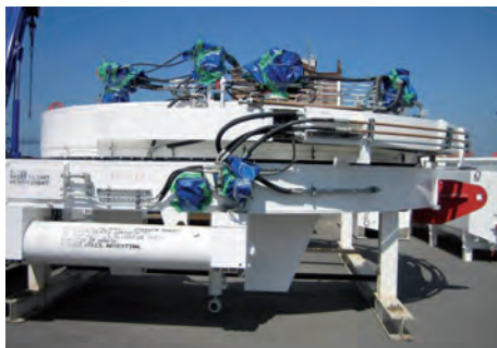
Figure 3: Segment erector after remanufacturing ready for final assembly in the TBM
