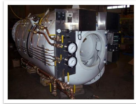
Figure 9. Man Lock for 7 bar pressure.
